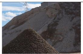
In the end, high-grade recycled building materials are produced. They are mainly used in road maintenance and construction, traffic road construction and earthwork.
